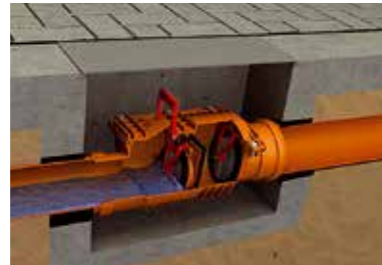
Blocked flap – backwater protection
