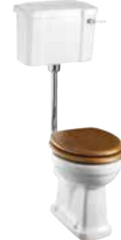
Standard low level WC with 520 rear entry lever cistern W 520 D 740 H 960-1140 Pan Height 420
